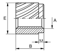
Female thread A = M2,5 Length B = 4.5 Min material thickness = 2.0 Outer diameter E = 5.3 Recommended bore diameter = 4.8
